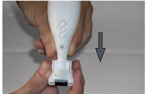
To install the new accessory, approach it to the Robomicro body, as shown in the picture, then push to fasten.
