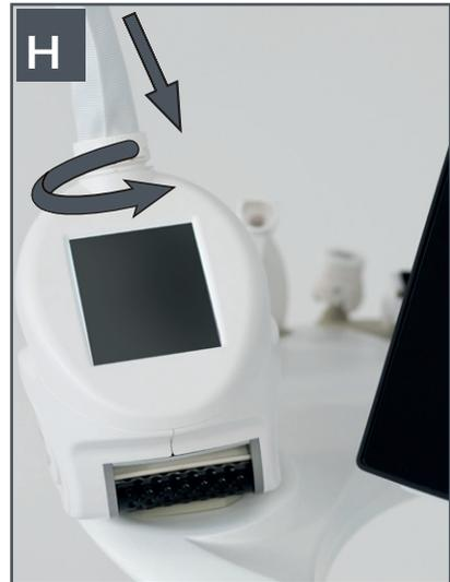
Remove the pipe, moving the nut away from the handpiece.
